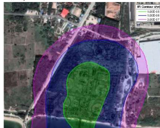
Figure 8.3 Individual Risk Contours for Nong Fab LNG Terminal (Process Area – Phase I + II)
