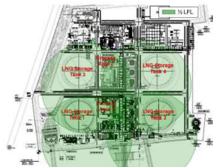
Figure 6.11 ½ LFL Contour for LNG Storage Tank Impoundment Pits
